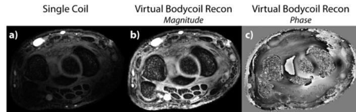
**Figure 3:** SENSE reconstruction of wrist images acquired on a 7T with an 8-channel coil array using the virtual body coil approach. a) An exemplary single coil image. b) The SENSE reconstructed magnitude image. c) The SENSE reconstructed phase image. Note that the virtual body coil approach results in a homogeneous intensity corrected reconstruction (b).
