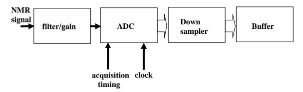
converter (ADC), which samples the analog NMR signal and converts it into digital format. Important characteristics of the ADC are its conversion bandwidth and resolution. The conversion bandwidth equals half the digitization rate. State-of-the-art ADCs such as the Analog Devices AD6645 allow conversion bandwidths of over 50 MHz at 14 bit resolution. Since NMR frequencies are generally well above 50 MHz, usually an alias of the NMR signal is detected.
