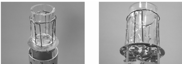
Figure 1: Photographs (top and bottom views) of the four coil phased array with impedance matching and decoupling networks.
