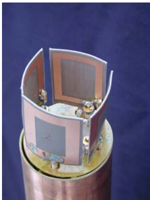
Figure 1: The four channel microstrip array coil
