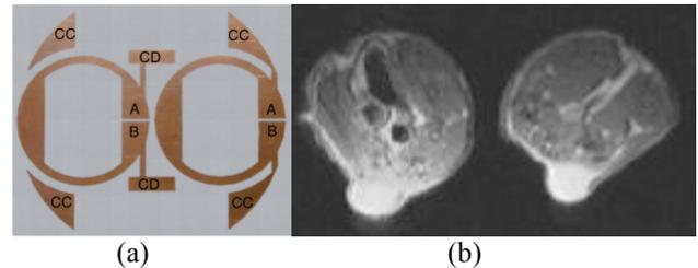
**Figure 2:** (a) A picture of the upper side of a 2'' by 1'' array cooled to 77 K for imaging shown in (b), CC and CD denote de-coupling and coupling capacitors, respectively, (b) axial slices (acquired simultaneously for two mice) of subcutaneous tumors present in a murine model of colon cancer.
