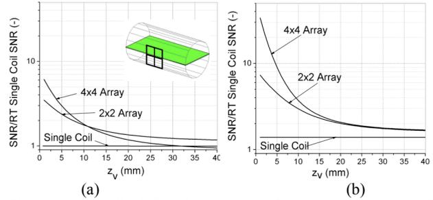
**Figure 1:** Normalized SNR improvement, for room temperature (RT) copper (a) and for HTS material (b), vs. voxel distance to the center of the array is shown.
